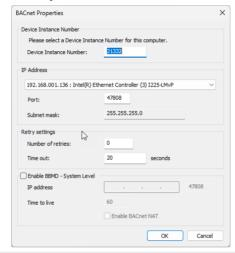
Note: If BACnet devices are on a different IP VLAN then an Enable BBMD – System Level option is available to bridge PC and BACnet devices networks.
