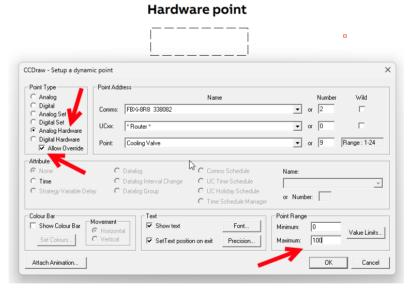
In addition, limits can be set for BACnet setpoints in the same way as they for **Unitron** points - as shown in the bottom-right of the screenshot above.
