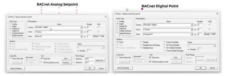
A Hardware Point can be Manually Overridden from a **Unitron Command Centre** Graphic and this is set up in **CCDraw** in exactly the same way as Unitron points - as shown in the screenshot below.
