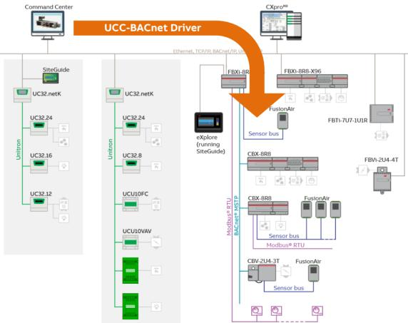
When Cylon BACnet devices are installed on a Site they must first be engineered in CXpro<sup>HD</sup>, and then when they are operational they can be added to the Unitron site as described below, and made visible within Cylon Engineering Centre (CEC) and Unitron Command Centre (UCC) alongside Unitron devices.
