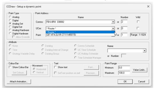
BACnet points from MSTP devices connected to an ABB Cylon Router are configured as below
